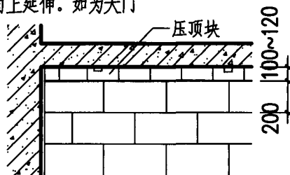
① 墙顶平砌压顶块
